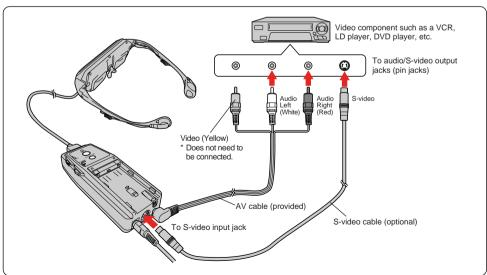
When the video component has more than one type of output jack, it can be connected with more than one Eye-Trek unit.
